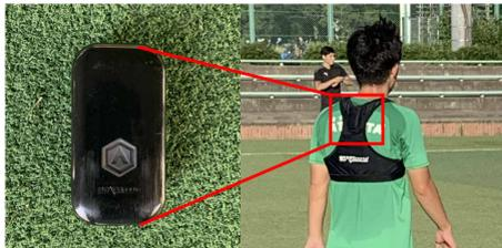
The device used for GNSS data collection
